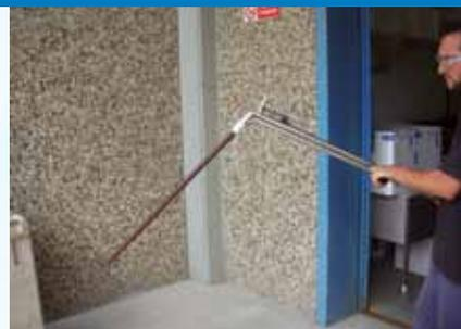
Coax gun with double interchangeable nozzle flat and cylindrical
